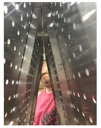
6. Next, place the double spacer over the screw and bring both pegboards together. The 2" screw should go through the center hole of the pegboard on the opposite side. Secure the pegboards together using an acorn nut.
