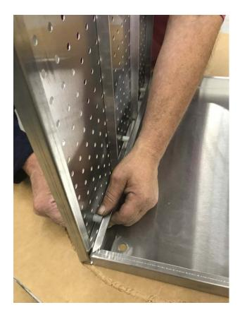
3. Attach the pegboard to the larger, bottom shelf. Line the shelf up with the bottom row of holes on the pegboard. Secure the pegboard to the shelf using acorn nuts. Acorn nuts should be on the outside of the pegboard.
