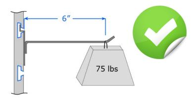
SlatWall  $MX^{TM}$  Strip can hold a 75 lbs point load hanging at a 6" distance from the slatWall face:
