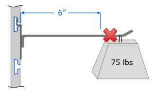
If the 75 lbs load moves further away than 6" from the slatwall face, the slatwall could break
