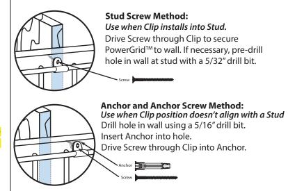
It's recommended to mount the PowerGrid™ on the wall with 2 or more Mounting Clips installed into studs. If you can only position the PowerGrid™ with Mounting Clips installing into 1 stud, use the Stud Screw Method to secure the Clip then use the Anchor method for the remaining Clips. All 6 Mounting Clips should be used to secure the PowerGrid<sup>TM</sup> safely and securely to the wall.
