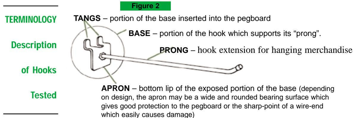
Pegboard hooks in common use vary widely in design. Figure 2 shows one basic type. Terminology used in Figure 2 may generally be applied to describe the four basic parts of any hook.
